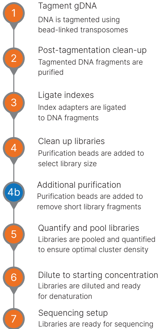
Figure 2: Modifying the Illumina DNA PCR-Free Prep protocol—An additional round of bead purification (step 4b) added to the protocol optimizes insert sizes and variant calling performance on the NovaSeq X Series.
