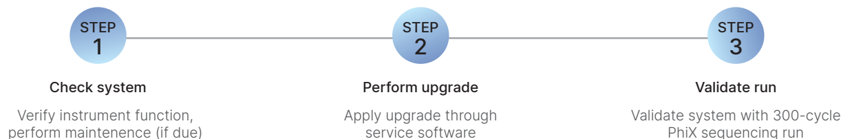
Figure 1: The NextSeq 1000 to NextSeq 2000 System upgrade process requires less than a day
