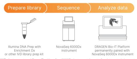
Figure 2: NovaSeq 6000Dx instrument workflow—The NovaSeq 6000Dx instrument is part of an integrated, three-step workflow that includes library preparation, high-throughput sequencing in either IVD or RUO Mode, and accelerated secondary data analysis with a paired DRAGEN Server.
